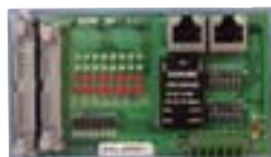
Local Input/Output Board (16 bits each for input and output)
