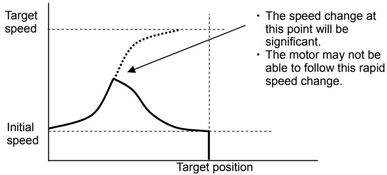
A speed pattern with a sharp tip is referred to as triangle driving.
