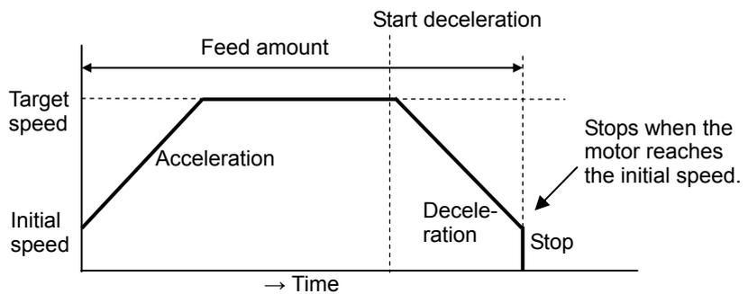
The appropriate deceleration start timing can be obtained easily from a calculation. The device can also set this position automatically. This deceleration start position is referred to as the rampdown point.
