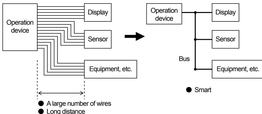
Historically, there have been a large number of wires for signal lines to connect equipment. By making the signals on these lines digital and putting them on a single cable, the number of wires decreases dramatically and it is much easier to maintain.
